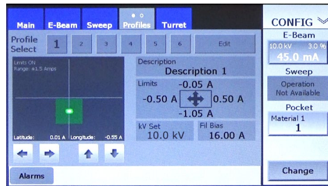
Figure 4-49 Profiles Page 1 After User Accepts the New Beam Position Interlock Limits
