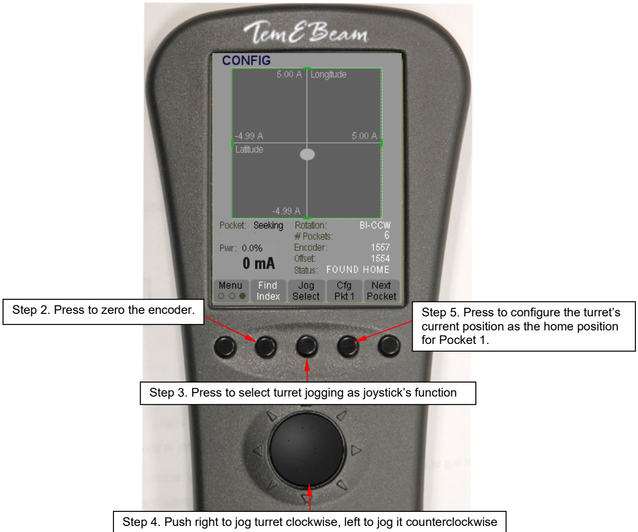
Figure 4-25 Using Config Screen's Menu 3 to Configure the Home Position for Pocket 1
