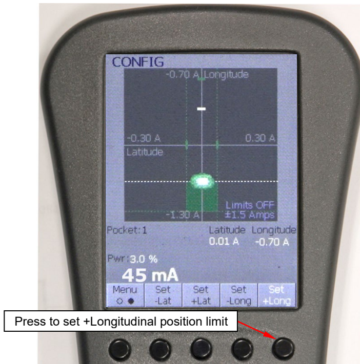
Figure 4-47 Remote Controller Screen After User Sets +Long Beam Position Interlock Limit
