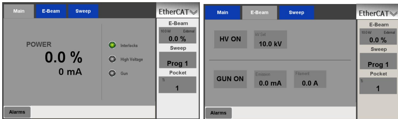
Figure 9-1 Appearance of Operations Mode Screens when All EBC Control Modules Are Configured as ETHERCAT
