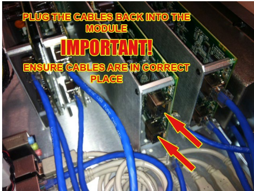
Figure 13-8 Plugging Cables into the New Control Module
