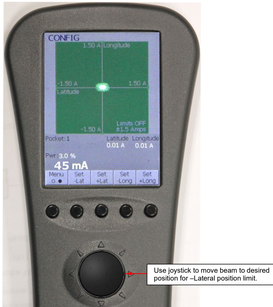
Figure 4-39 Remote Controller in Config Mode, Beam On at 5%, Menu 2 Displayed
