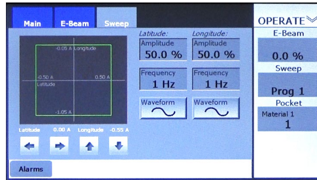
Figure 4-50 Operations>Sweep Screen After Beam Position Limits Are Set
