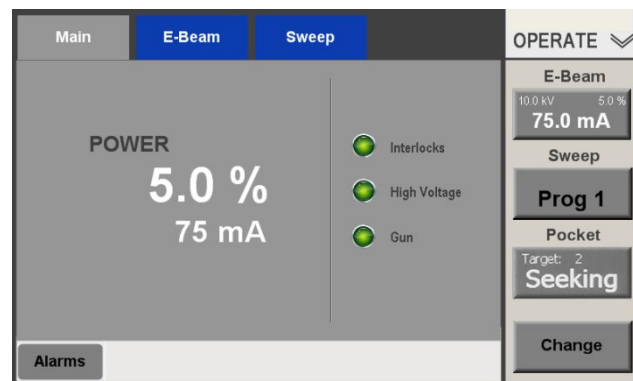
Figure 2-17 Pocket Button When Turret Is Rotating
