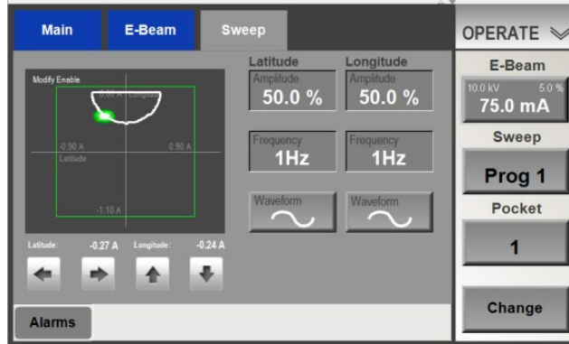
Figure 5-8 Ops&gt;Sweep Screen with Beam Sweep Displaying the 'Clipping Effect'
