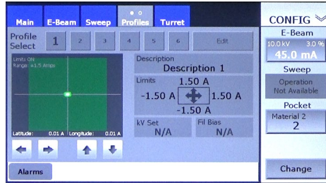
Figure 4-37 Profiles Page 1, Beam On at 45 mA
