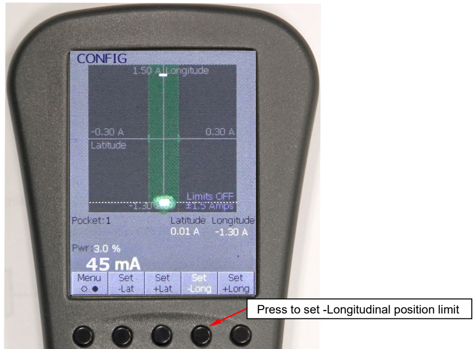
Figure 4-45 Remote Controller Screen After User Sets -Long Beam Position Interlock Limit
