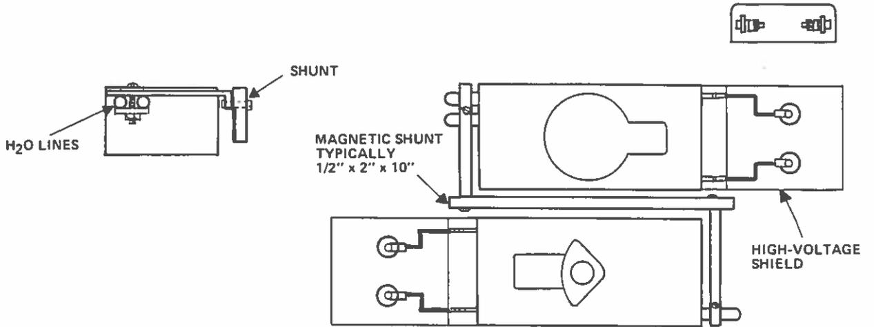
Figure 3. Schematic diagram of a typical chamber layout using two sources
