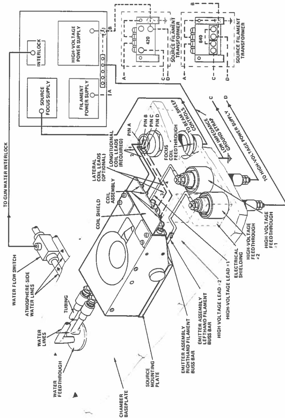
Figure 2. Installation details and interconnect block diagram for the SFIH-270-2
