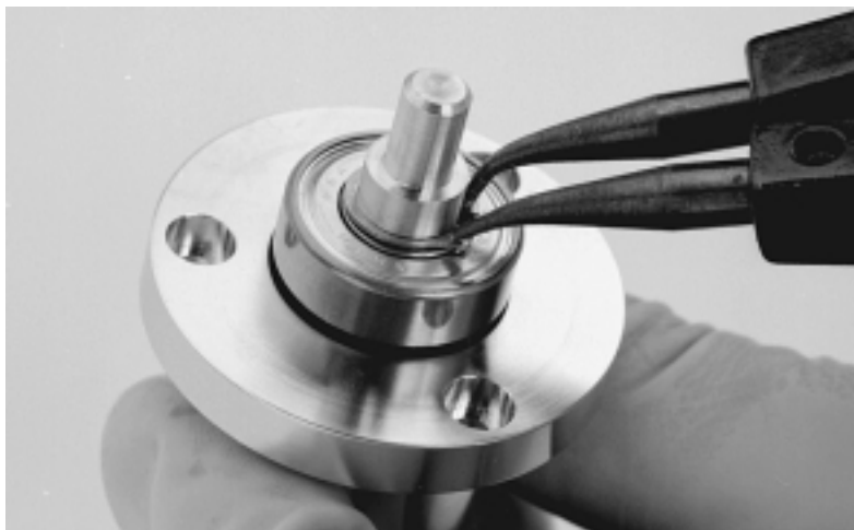
Figure 5-31. Removing the retaining ring that retains the drive shaft
