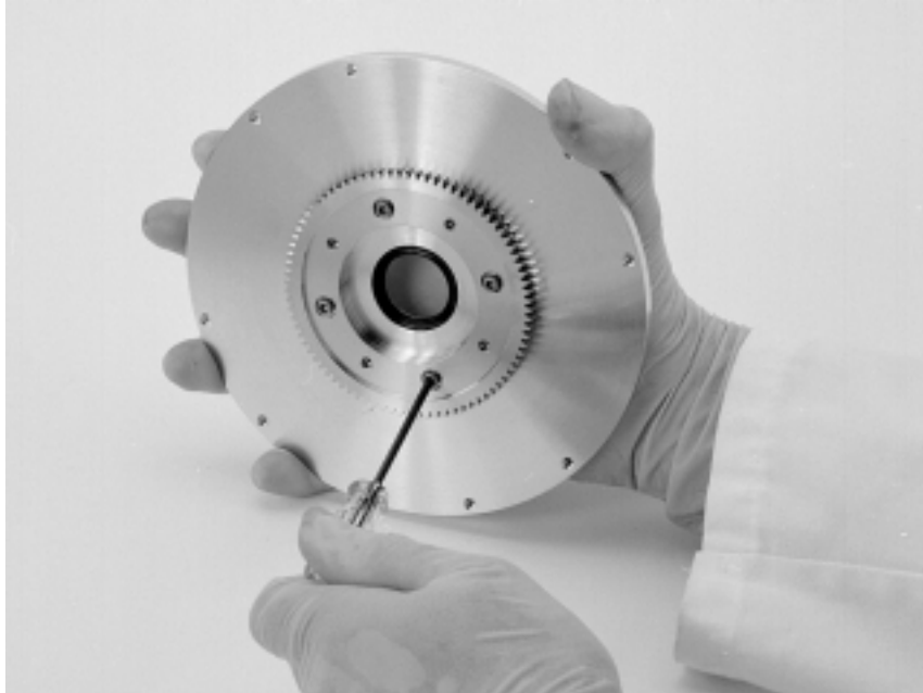
Figure 5-25. Removing the ring gear from the crucible mounting flange
