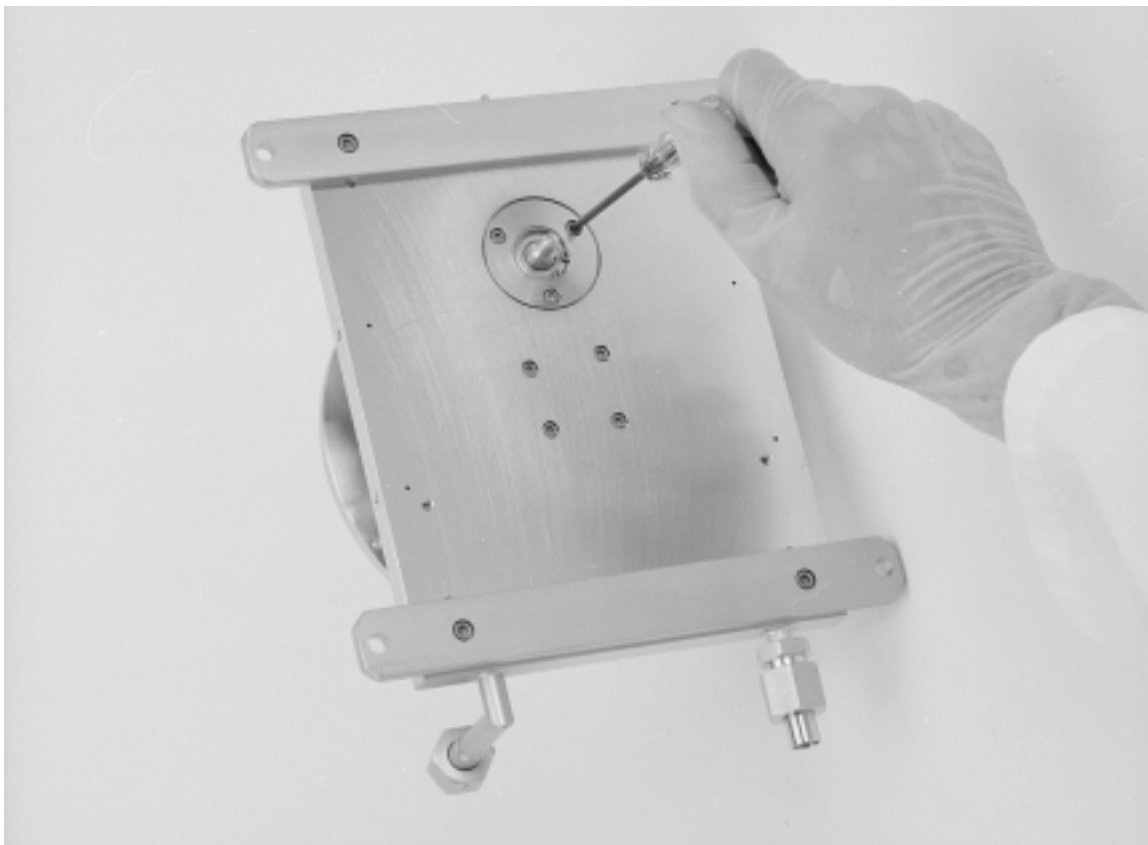
Figure 5-21. Detaching the drive shaft
