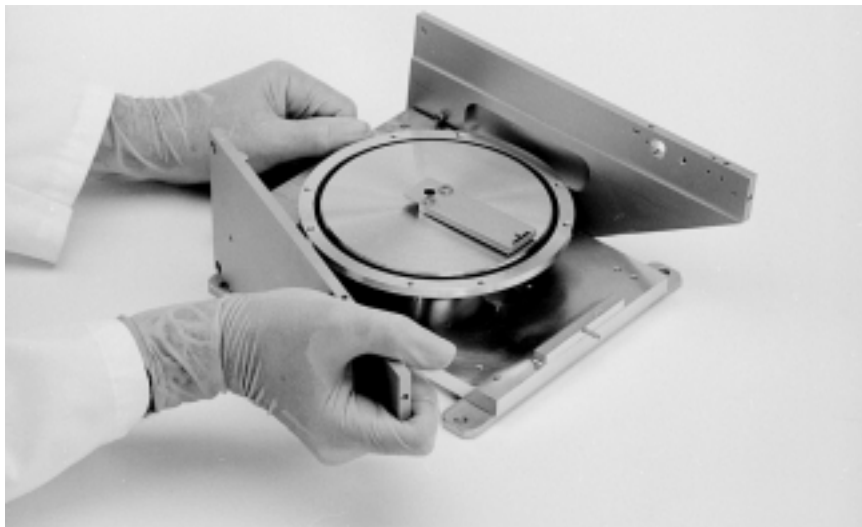
Figure 5-18. Correct technique for detaching pole pieces from magnet and base plate
